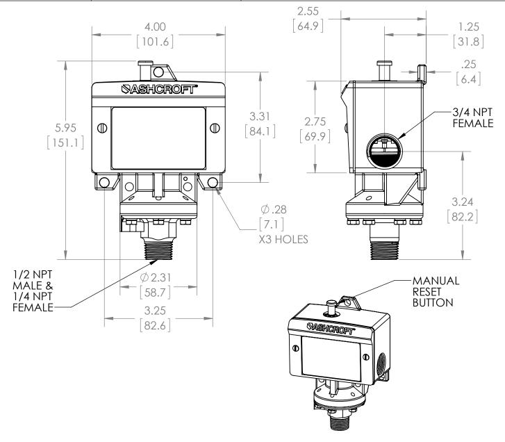
NOTE: SWITCH CODE 28 IS FOR MANUAL RESET TRIP FOR INCREASING PRESSURE.
